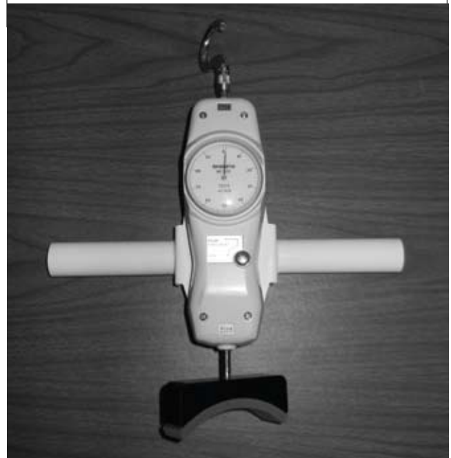
FIGURE 1. Force Gauge for Strength Test
